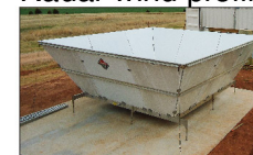
Radar wind profiler
