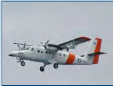
The CIRPAS Twin Otter is a non-pressurized turbo prop twin-engine aircraft that will operate at an air speed of about 100 knots during RACORO science flights.
